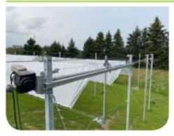
The unique drive design powers the roof covering at the peak and valley to ensure optimal closure of the roof covering. (Patent pending)
