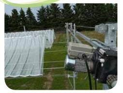
One motor can close 0.8 ha or 2 acres of roofs in 4-6 minutes allowing for rapid protection of crops. The straight drive line avoids the need for universal joints.
