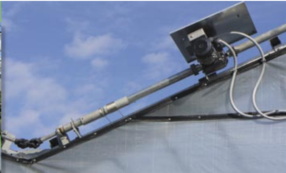
Direct drive uses heavy duty U joints
